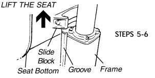
FIGURE 1 - REMOVING THE SEAT
